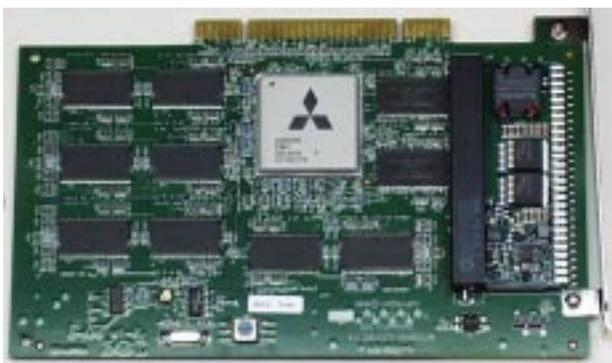
Figure 5: A picture of the Mitsubishi Electric Cube-4/VolumePro board with the vg500 rendering chip.
